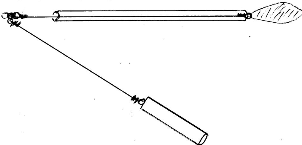
Dowel leader to be a minimum of 25 kg maximum of 50 kg breaking strain and shall be no less than 230 mm long.
